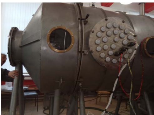
Fig. 27 Connect the technological cables with the control board and infrared regulator device
