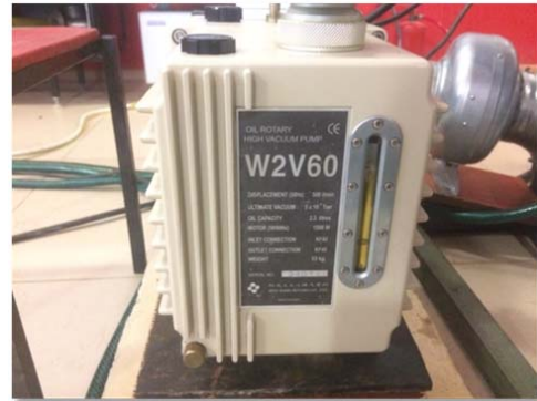
Fig. 18 Rotary high vacuum pumps Model W2V60
