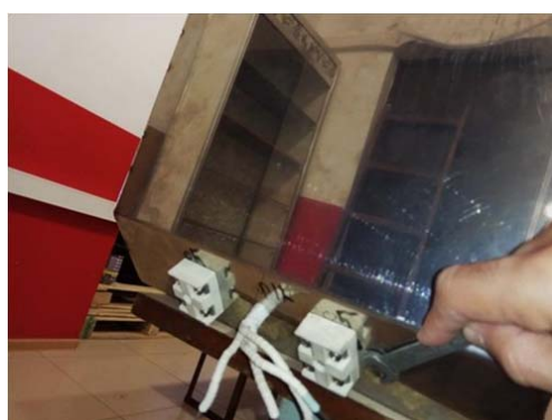
Fig. 21 Fixing infrared lamp
