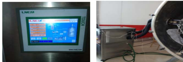
Fig. 29 Connect the refrigerator cables to the cold plates
