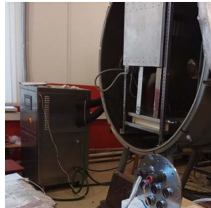
Fig. 14 Cooling system for the MVC
