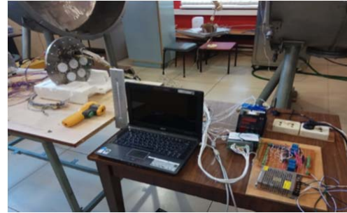
Fig. 28 Connection of the computer with a data acquisition system and onboard control unit
