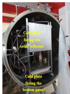
Fig. 24 Adjust the cooling plates and refrigerator temperature
