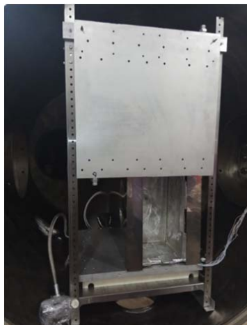
Fig. 20 Fixation of the cooling plate
