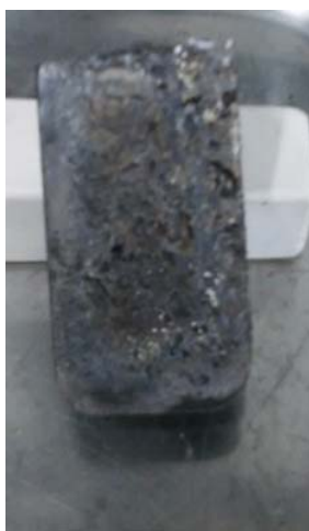
Fig. 2 Aspect of U-5wt.%MO ingot
