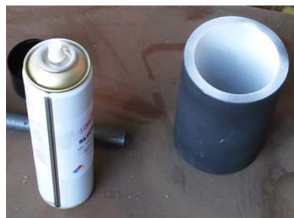
Fig. 1 Graphite crucible coated with boron nitrite
