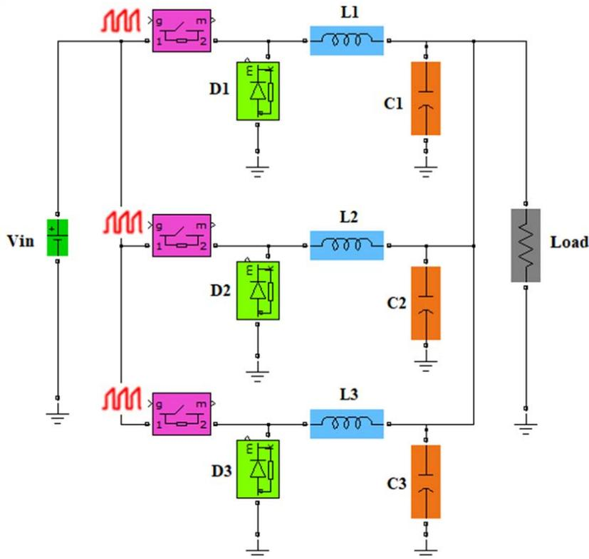
Fig. 2 Three-cell Buck converter associated in parallel
