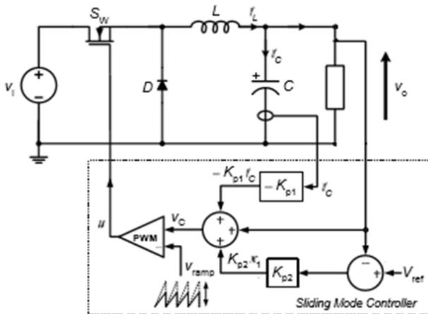
Fig. 3 PWM-based SM control scheme
