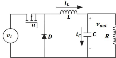
Fig. 1 Basic topology of the Buck converter
