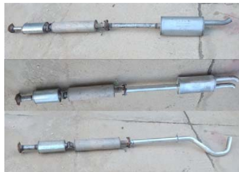
Fig. 2 Construction of the expansion chambers
