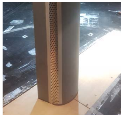
Fig. 7 Model showing porous plate covered suction section
