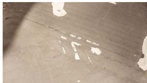
Fig. 11 Mold surface cracking between beads
