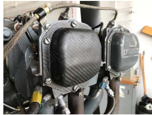
Fig. 14 Test fitting of carbon fiber valve cover
