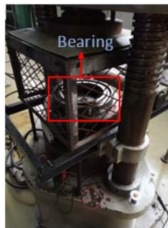
Fig. 6 Industrial force compression machine
