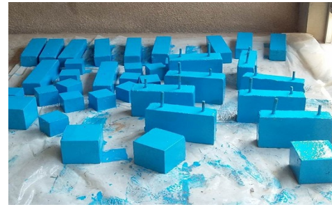
Fig. 2 Epoxy coating for the concrete specimens
