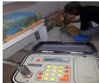
Fig. 10 Electrical resistivity measurement
