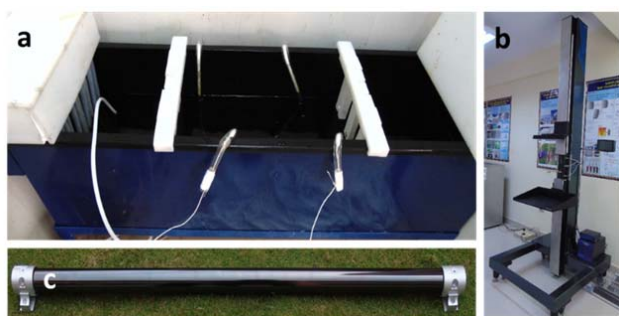
Fig. 5 (a) Chemical bath reactor (b) Dip coater and (c) ARCI's indigenously developed 1m receiver tube
