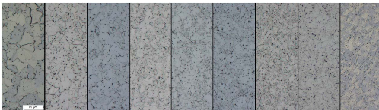
Fig. 3 Evolution of the microstructure of titanium grade 4 wire shown at the centre of its transverse section; wire diameters from left: 8.13, 7.18, 6.48, 5.87, 5.22, 4.73, 4.25 and 3.81 mm
