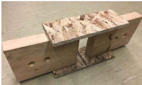
(b) Typical joint test specimen
