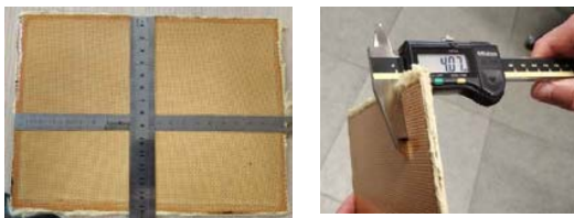
Fig. 23 The dimensions of Kevlar ® plate produced for this study
