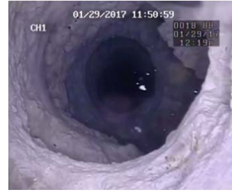
Fig. 8 Recording acquired during CCTV camera logging – cavities in recharge zone
