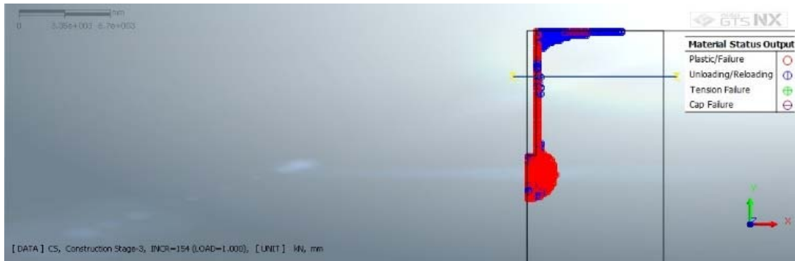
Fig. 34 Finite element results of the Formed plastic points under load of 3250 kN (Failure load)
