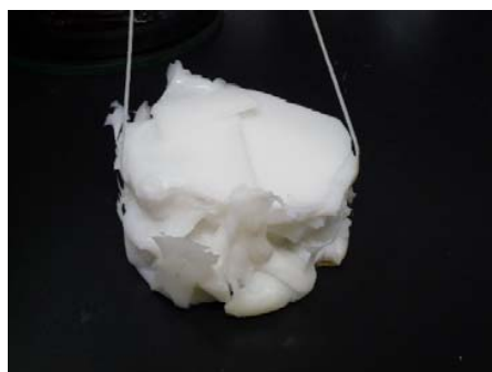
Fig. 2 Molten polyethylene container after heating
