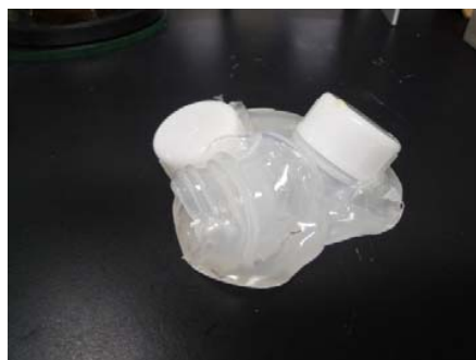
Fig. 1 Molten polypropylene bottles after heating
