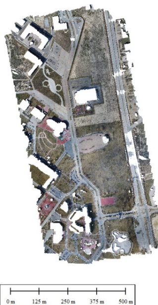
Fig. 3 Point cloud filtered by CSF (Ground point)
