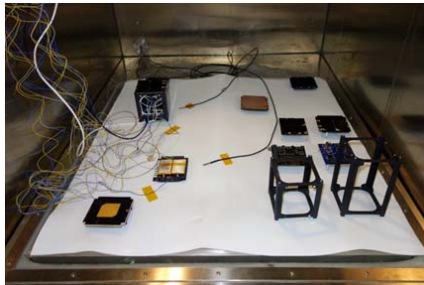
Fig. 4 CubeSat and modules in the climatic ATT Climatic chamber CH 2000
