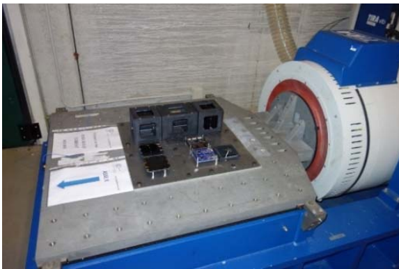
Fig. 8 CubeSat and modules installed on TIRA Shaker
