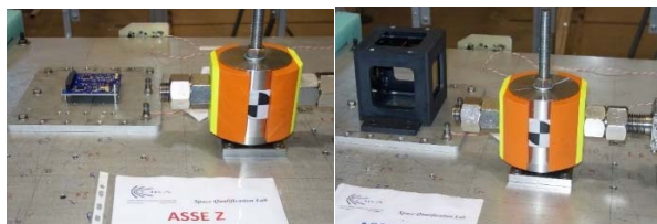
Fig. 13 CubeSat and modules installed on ringing plate of shock facility. Vertical axis
