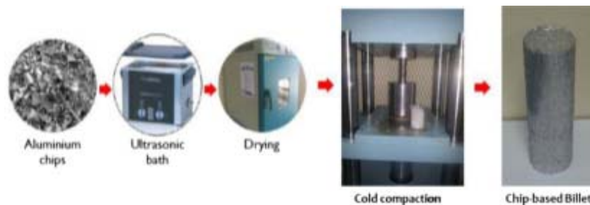
Fig. 2 Preprocessing of chips before consolidation
