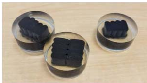
Fig. 3 Polished microscopy specimens
