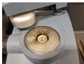
Fig. 8 Specimen loaded in DSC's chamber
