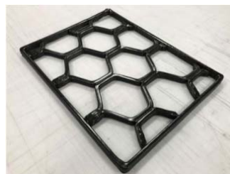
Fig. 1 Prototype 3D printed recycled carbon fiber part
