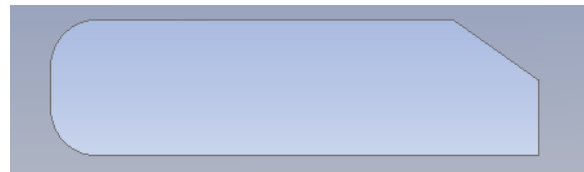
Fig. 1 (b) An idealized physical model of Ahmed body (Corresponding to Fig. 1 (a))
