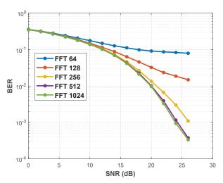
Fig. 7 BER for different FFT size N with QAM=64 and L=6
