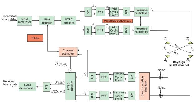
Fig. 2 Simplified block diagram of MIMO-OFDM system
