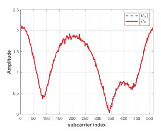
Fig. 5 Difference between the ideal and the estimated channel frequency response for the channel  ${\cal H}_{11}$
