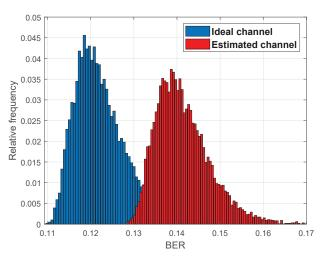
Fig. 12 Relative frequency distribution of the BER with ideal and estimated channel resulting from 10000 Monte Carlo trials with QAM=64,  $N=256,\,SNR=10dB$  and L=6
