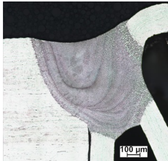
Fig. 9 The macrostructure of the EB welded joint
