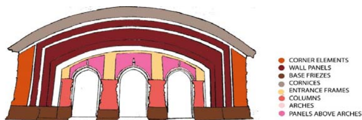
Fig. 28 Schematic Triple-entrance Façades
