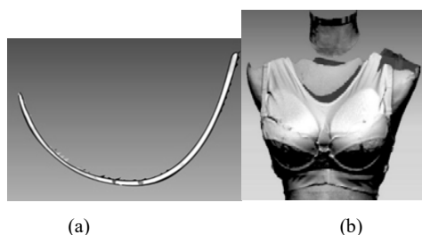
Fig. 3 3D scanned image of (a) planar underwire, (b) soft breast manikin with donned bra
