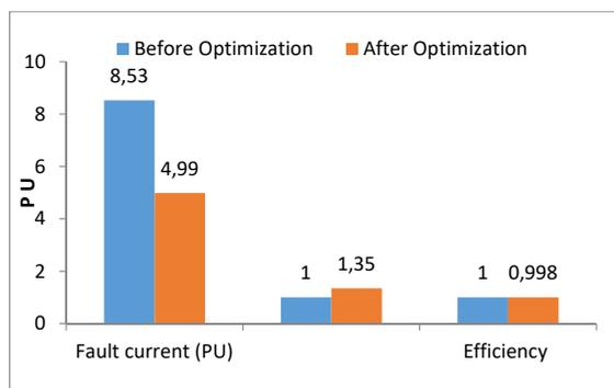
Fig. 7 Fault current reduction optimization
