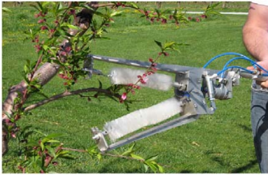
Fig. 8 Prototype end effector for automated blossom selective thinning [25]
