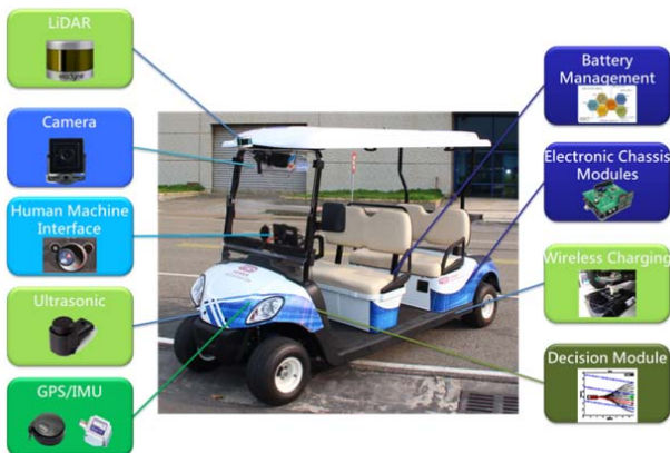
Fig. 8 The in-house built self-driving e-golf cart
