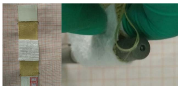
Fig. 11 \text{Al}_2\text{O}_3 aerogel/fabric flexible materials
