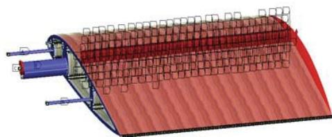
Fig. 3 Boundary conditions applied to morphing structures
