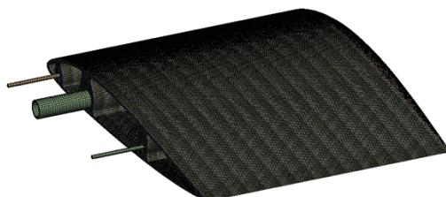
Fig. 4 Applied mesh to a wing model
