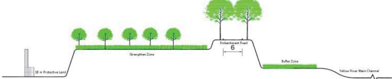
Fig. 30 Section view of a Yellow River embankment. Repainted from Yellow River Authority
