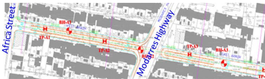
Fig. 6 Plan of bore holes (BH) and test pit (TP) locations (red marked points)
