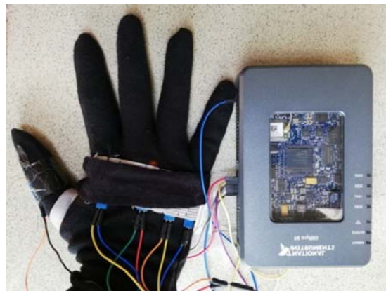
Fig. 2 Gesture digitization glove assembly
