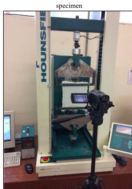
Fig. 6 Setup of testing Poisson's ratio
