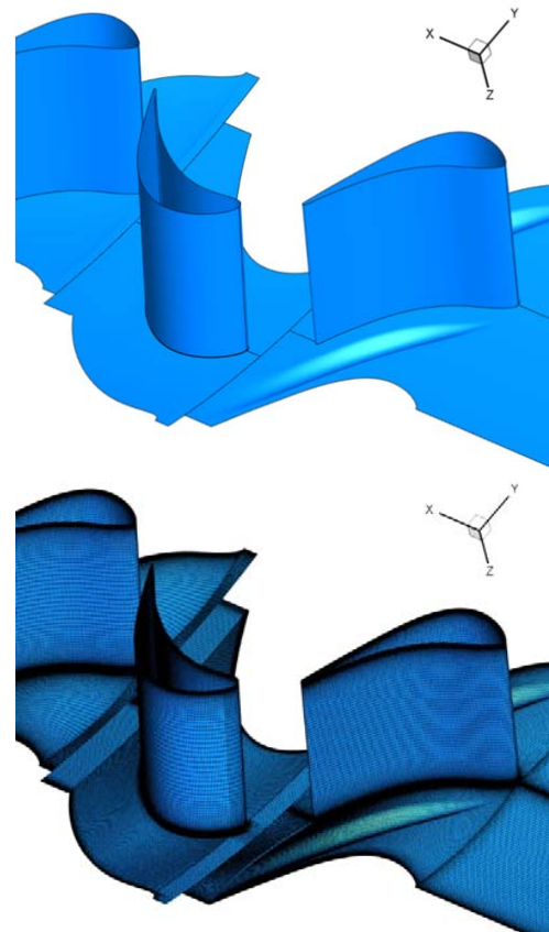
Fig. 4 Non-axisymmetric optimized casing design imported in ICEM CFD
