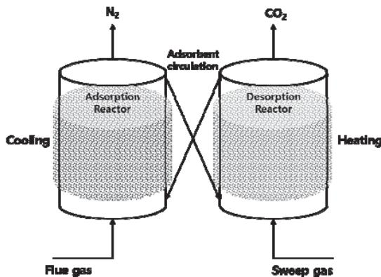
Fig. 1 CFB riser for carbon dioxide capture
