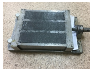
Fig. 5 Standard mortar prisms for testing of pozzolanic activity
