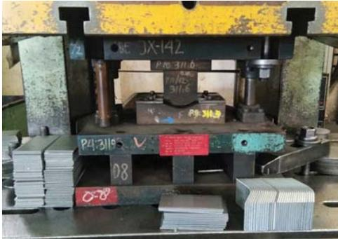
Fig. 3 Conventional die unit (courtesy of PT.SPI)
