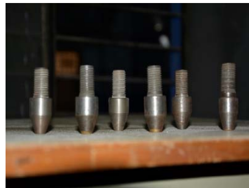
Fig. 8 Nozzles made of WC and HCHC steel
