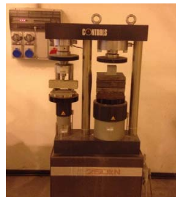
Fig. 4 Photograph of the test frame with twin columns used in the experimental campaign for the compressive and indirect tensile tests
