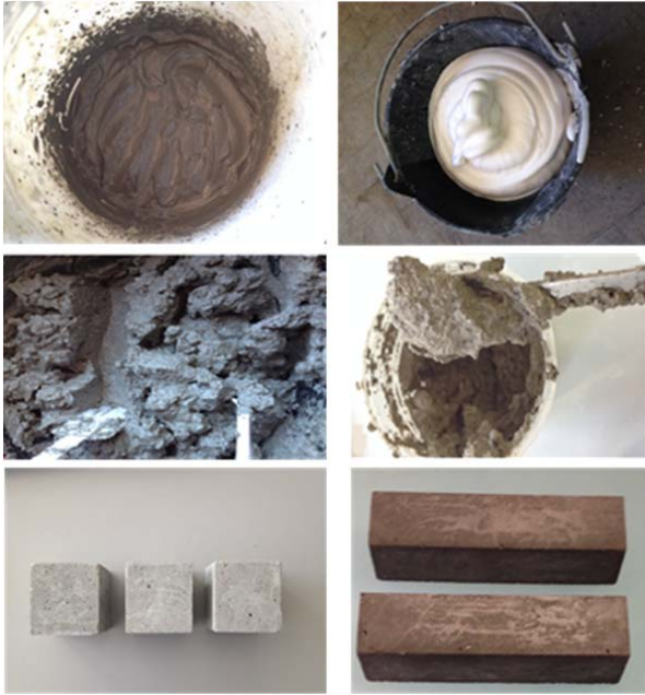
Fig. 1 Preparation of extrudable foamed concrete specimens
