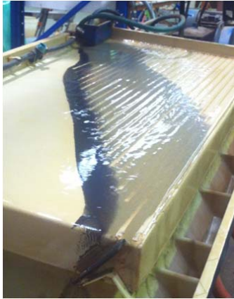
Fig. 6 Wilfley Table, low gravity stage (2 0 ) of processing
