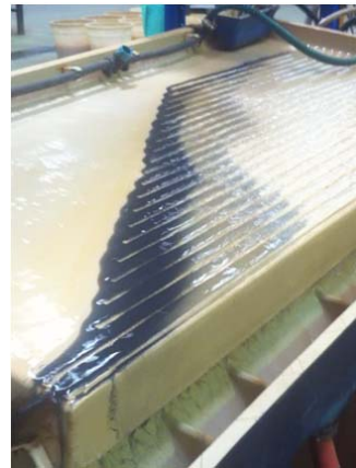
Fig. 7 Wilfley Table, High gravity (6 0 ) stage of processing
