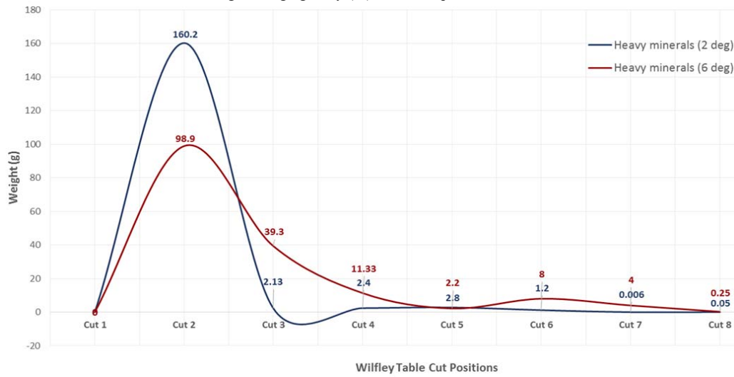
Fig. 11 Comparison of high & low gravity heavy mineral separation
