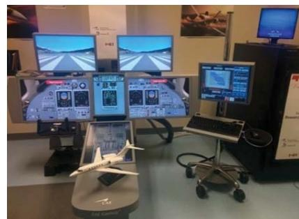
Fig. 1 Cessna Citation X Research Aircraft Flight Simulator (RAFS)
