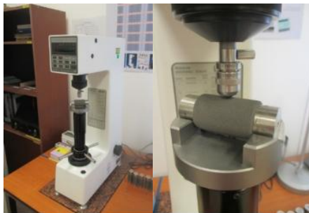
Fig. 4 Used Hardness Tester LECO LR-300TDL
