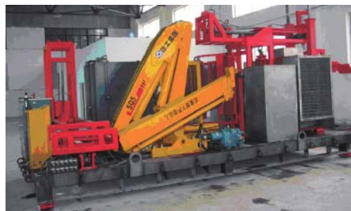
Fig. 1 The prototype of the curved plane oil skimmer system
