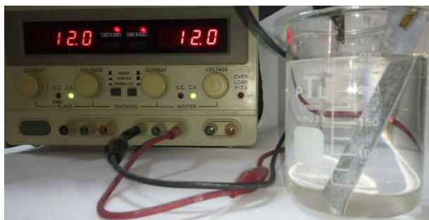
Fig. 3 Anodizing of Aluminium in 12 wt.% Phosphoric acid at 12V
