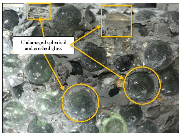
Fig. 10 The fracture surfaced appearance of concrete with spherical and crushed glass as coarse aggregate
