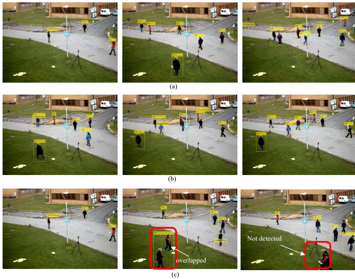
Fig. 3 Experimental results of the Scene2 on the unorganized scene of pedestrians walking in different directions. (a) and (b) Correct detection and tracking. (c) Failure cases happened when pedestrians are moving close to each other
