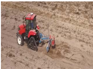
Fig. 8 Building bumps and hollows using a plough
