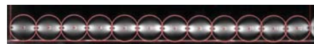
Fig. 18 One dimensional chain of photoelastic particles with marked circular boundaries of particles
