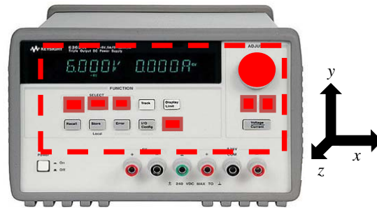
Fig. 8 Power supply control areas
