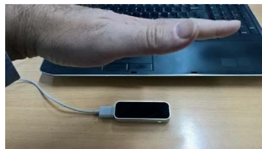
Fig. 6 Leap Motion controller use
