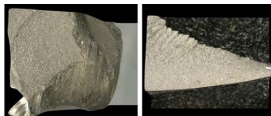
Fig. 13 Fracture of carbide bit
